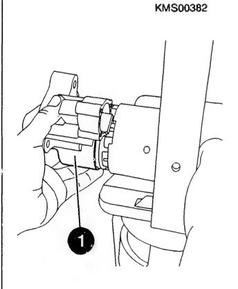
STARTING MOTOR ASSEMBLY Assembling drive-end bearing Slacken off clamping support, re-check correct positioning (marks) of drive-end bearing and commutator end shield and secure. Bolts (1) must run in parallel with imaginary center axis of starting motor and be tightened alternately and evenly. Use torque wrench. Torque wrench: Comm. avail. Tightening torque: 5,5...6,0 Nm
